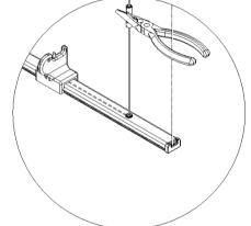
To loosen the steel wire, place the regulator pin on the bottom rail and press down-as shown in Drawing 2.
